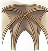
RIBBED VAULTS (Óveda de Cruceria) Intersecting vault system distributed weight efficiently, allowing for higher collings and thinner walls.
